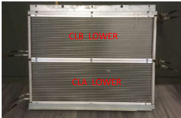
LOWER BLOCK GAS COOLER FRONT SIDE
