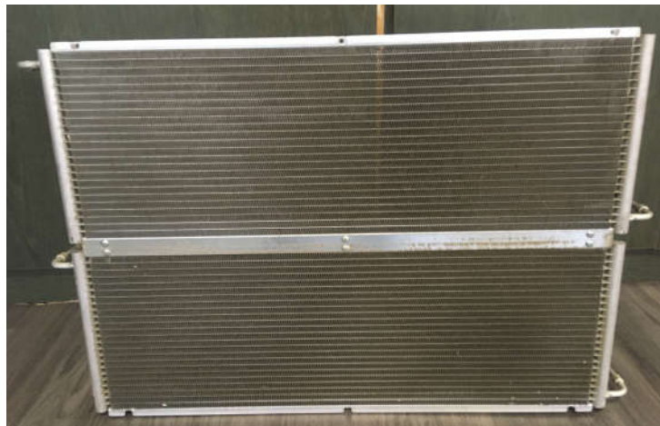
Bloc Gas Cooler assembled
